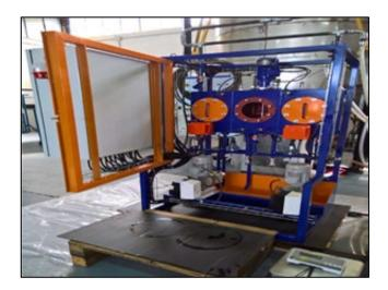
Using the COBU unit, a ship entering an ECA can match the BN in the cylinder oil to the 0.10%S fuel within 2 to 3 hours and all at the touch of the tabs on a touch screen. This simplifies BN changeover for ECAs, optimises performance and cost of cylinder oil when the BN is matched to the fuel Sulphur content.
