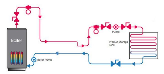
An Application of a Thermal Oil System: Maintaining the Temperature of Product Storage Tanks
