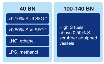
\* Some OEMs recommend the use of up to 70BN for fuel oils with with <0.5%S (such as, ULSFO and VLSFO). We believe it would be prudent to include this caveat: "when excessive residues on piston top lands are observed, adjust the cylinder oil feed-rate and/ or re-select cylinder oil".
