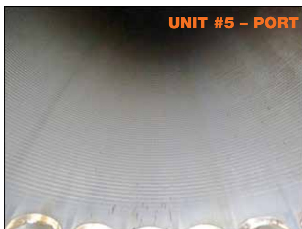
Honing marks were visible which indicates satisfactory condition. No abnormality was observed.
