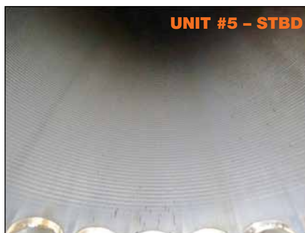
Honing marks were visible which indicates satisfactory condition. No abnormality was observed.
