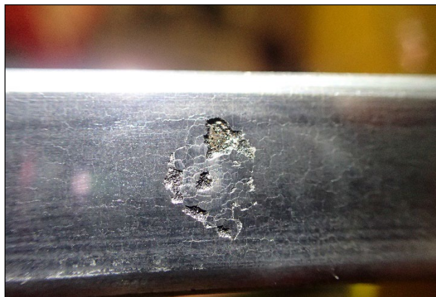
The pictures above show flaking/peeling of piston ring coatings
