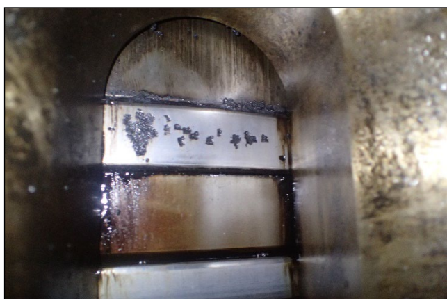
The pictures above show flaking/peeling of piston ring coatings
