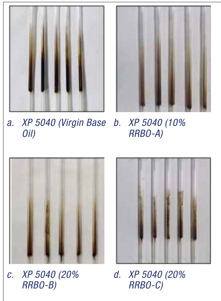
Fig. 2 Komatsu Hot Tube (KHT) test results comparing deposit formation for XP 5040 formulations with virgin base oil and RRBO blends.
