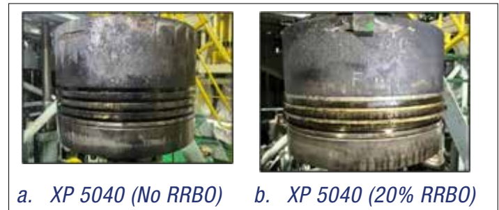
Fig. 7 Piston condition after 3891 hours of operation with XP 5040 formulations using virgin base oil and a 20% RRBO blend.
